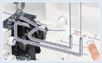
**RevolutionAir**™ with Tubular Loopers allows you to thread in any order and avoid tangles and knots as threads are not exposed.
